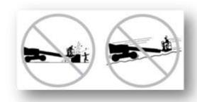
It shall limit the travel speed according to the ground condition, crowdedness, slope grade, person position and other possible factors may cause crush accident.
