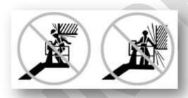
Beware of the danger of being squeezed when gripping the guardrails of the platform.
