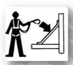
Every person to enter the platform shall wear the safety belt or use other security devices in accordance with the governmental regulations. And all the lacing wires shall be tied at some fixed points on the platform.
