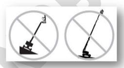
Do NOT regard the tile alarm as the level indicator. The tilt alarm on the platform will sound when the machine is severely tilted..
