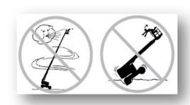
\* When stowed, it shall be driven extremely carefully and slow down the drive speed on the uneven or steep slope areas, unstable or slippery ground with gravel or near the cave, etc.
